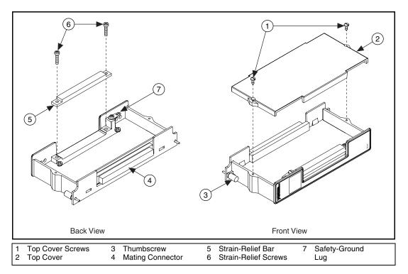
Figure 1. SCXI-1314 Parts Locator Diagram
